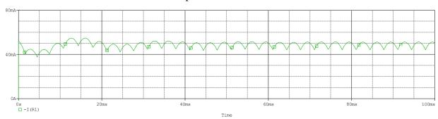
Three Phase Full Wave Rectifier Output Current:
