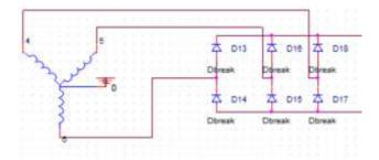
Three Phase Full Wave Rectifier Output Voltage:
